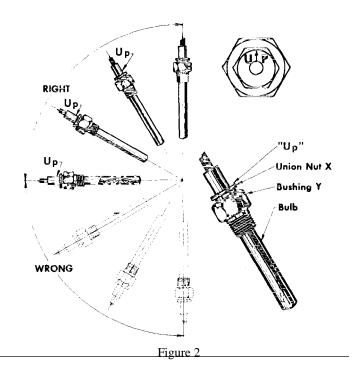
CAUTION: Do not place capillary on or near steam, hot oil, exhaust manifold or surfaces which have a temperature that would affect the operation of the instrument. Avoid unsupported lengths of capillary. Do not use the capillary as a support for other objects. Excessive lengths of capillary should be coiled and well supported. Avoid bending or twisting capillary at the connection between the bellows cup or the bulb assembly.
